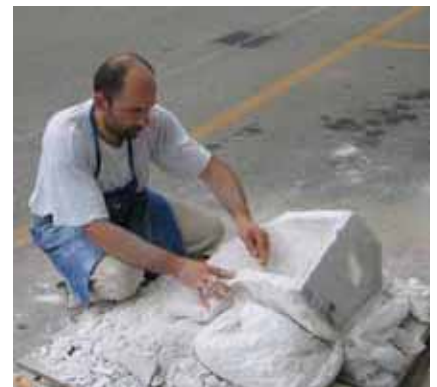
Opening forms and cleaning the glass pieces.
