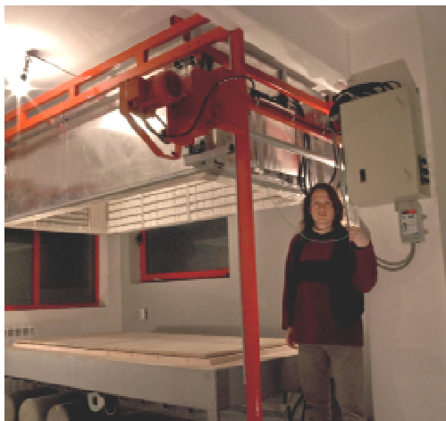
The inside measures: 110/240cm, 60cm high . It opens up by an electric motor. An interesting feature is the fan underneath that pushes in air through the bottom elements which is very useful for drying moulds. The configuration of the elements allows me to turn on and off any of the 3 zones manually. Thermo-controller is 'Bentrup TC-507'.
