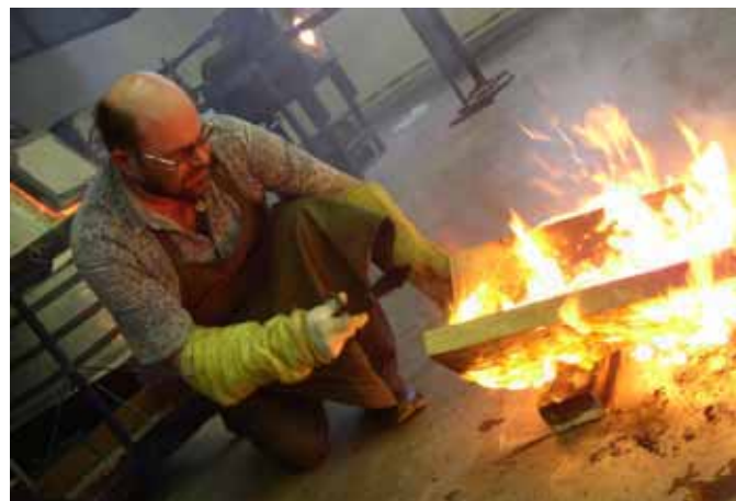
Glass casting in wooden mould. Remigijus Kriukas Photos made by INDRĖ STULGAITĖ KRIUKIENĖ.
