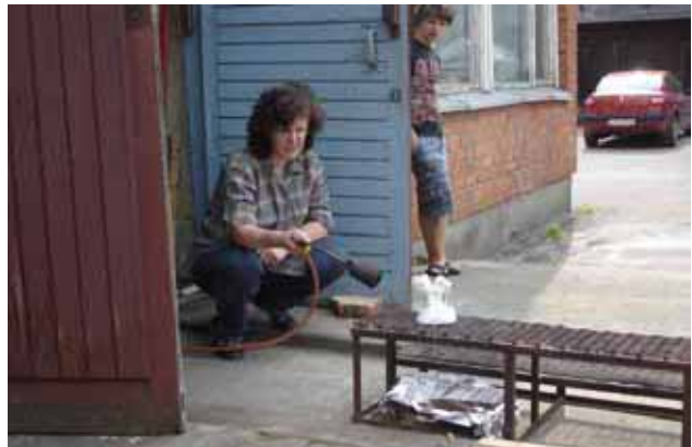
Burning out the wax models from the Luminar mold mix molds before kilncasting. Mare Saare.
